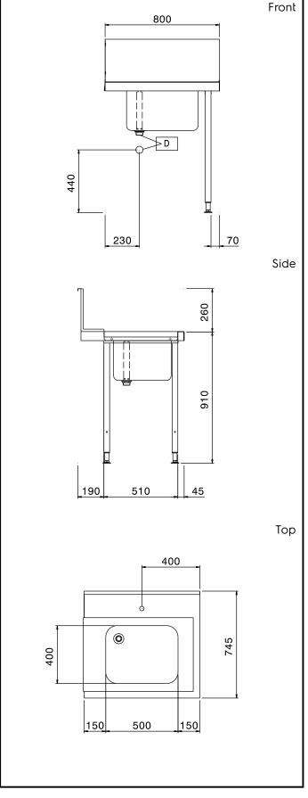
Handling System for Hood type Pre-wash Table with Bowl Right to Left, 800mm
